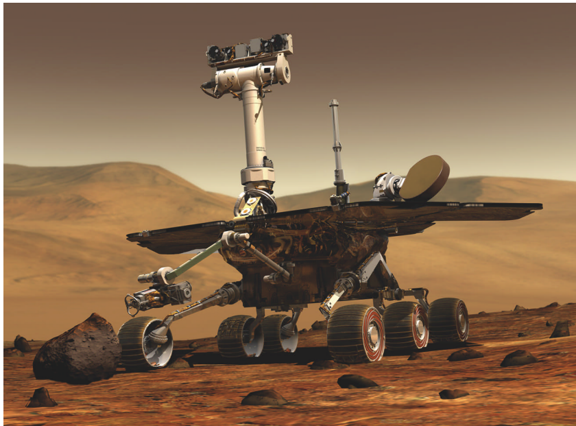
The Instrument Deployment Device, or IDD, is an Alliance Spacesystems robotic arm that brings the scientific instruments on NASA's Mars rovers into contact with rocks and soils on the planet. Courtesy of Alliance Spacesystems.
