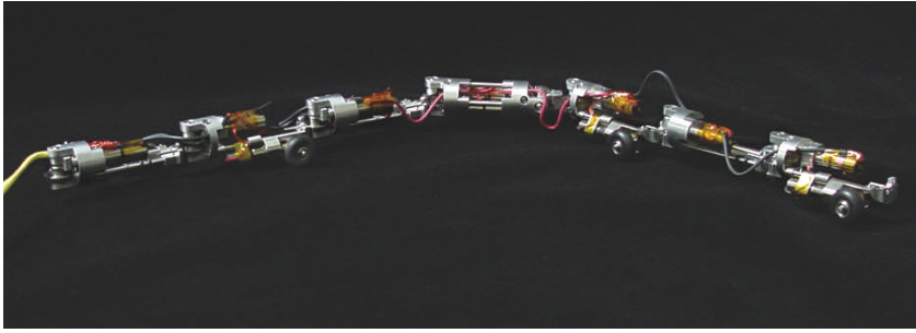
The GPEX gas-pipe explorers are a series of self-propelled prototype robots. Where the first GPEX model moved like an inchworm to inspect 4- and 6-in. underground natural gas pipes, the latest design contains deployable wheels and can access pipelines via a hole as small as 1 in. in diameter. Courtesy of Alliance SpaceSystems.
